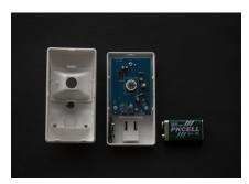
3. Take out the old battery and replace it with a new 9V battery
