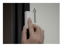
2. Push the door sensor up to remove it from the frame
